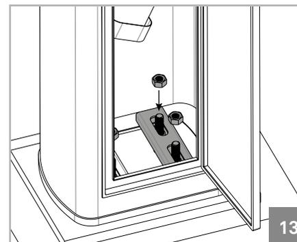
**3•** Place the fastening metal plates and fix the barrier to the ground tightening the nuts supplied with the product.
