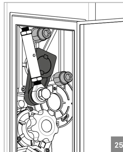
The mechanical stoppers shown in the image on the side, were developed to limit the movement of the arms inside the barrier's body.
