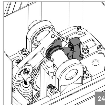
The mechanical limit-switches of the barrier are shown on the image on the left. They consist of two rings fixed to the boom's rotation shaft, that when opening or closing will activate the micro-switches also installed. This will cause the control board to stop the barrier when the micro-switches are activated, one for each type of maneuvers.
