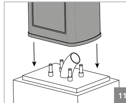
**01•** With the bolts already fixed on the cement foundation, respecting the dimensions of point 2, place the barrier on top of the foundation in a way that the screws stay inside and centered with the barrier.
