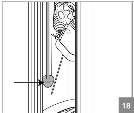
**02•** Rotate the rod (image above) to unlock the cover. There are two rods, one on each side of the barrier.
