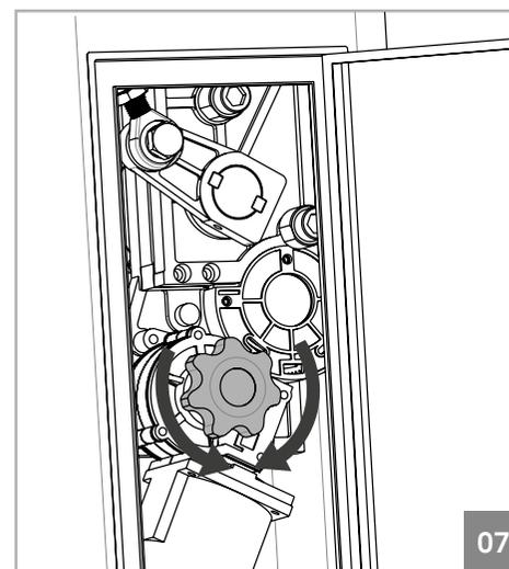
**02•** The unlocking is made by pressing and rotating the motor wheel shaded on the image on the side. The rotation direction to unlock will depend on the current stage of the boom (opened or closed) which will make the rotation possible to only one side.
