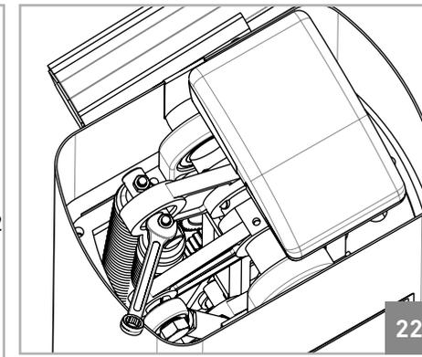
**ADJUSTMENT•** To adjust the springs, you must use a wrench to fasten or release the springs nuts. If you rotate them clockwise you are giving tension to the springs causing the boom to rise up, and rotating counterclockwise you are removing tension from the springs causing the boom to descend.
