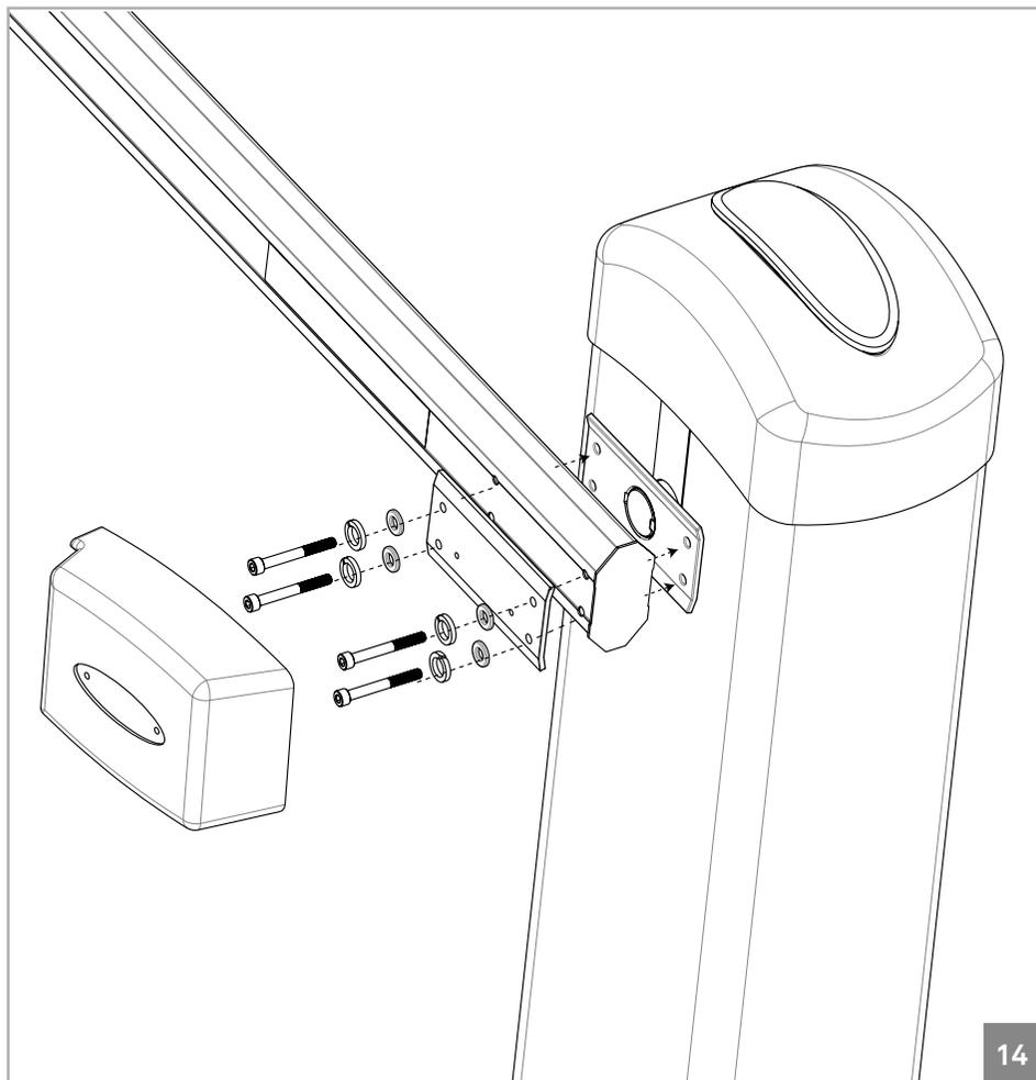
To assemble the boom, you must place the boom on the barrier fixing plate and align the four holes on each piece. Then you just need to place the boom fastening metal plate and use the screws to fasten the three parts together. When the boom is fixed, use the cover to hide these fastening parts.
