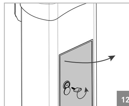
**02•** Open the door using the key to unlock it, and pull it to the outside.
