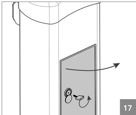
**01•** Open the door using the key supplied to unlock it and then pull it to the outside.
