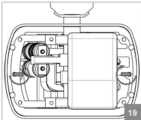
**03•** The hooks that secure the top cover are also rotated and release the cover.
