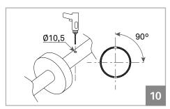
**01** • Effect on the tube of the shutter a pas sing perforation Ø10 perpendicular to the axis.
