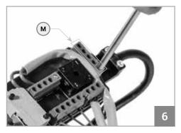
17 • Connect the terminal block (M) of the power wire to the limit switch respecting the right direction (figure 6). Fasten the terminal block through the four screws.
