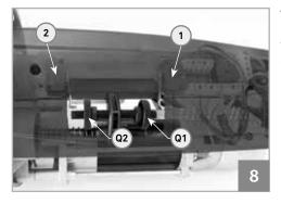
19 • After having installed the mechanical parts and electrical connections, proceed to the regulation of the limit-switches as shown in figure 8.
