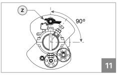
**02** • After assembled the two elements of the gearmotor (G), check that the pawl (Z) is in the highest position perpendicular to the rolling shutter axis.
