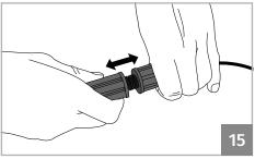
To unlock the motor simply unscrew the unlocking piece at the end of the steel cable by turning it to the left. To lock the engine again, tighten the same piece.
