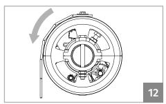
03 • The downward run of the roller shutter shall ben consistent with the downward run of the safety brake. Place the gear motor as shown.
