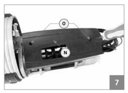
18 • Close the limit switch through the plastic cover (N) and then fasten with the two screws (0), checking the correct disposition of the cables (figure 7).
