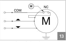
**04** • For microswitch versions, connect the micro switch's cable (W) in series to the fee ding cable (common) of the gearmotor.
